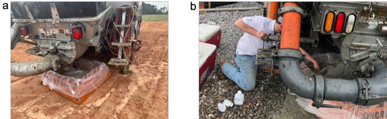
Fig. 2. (a) Portable Washout Box and (b) Sample Collection
