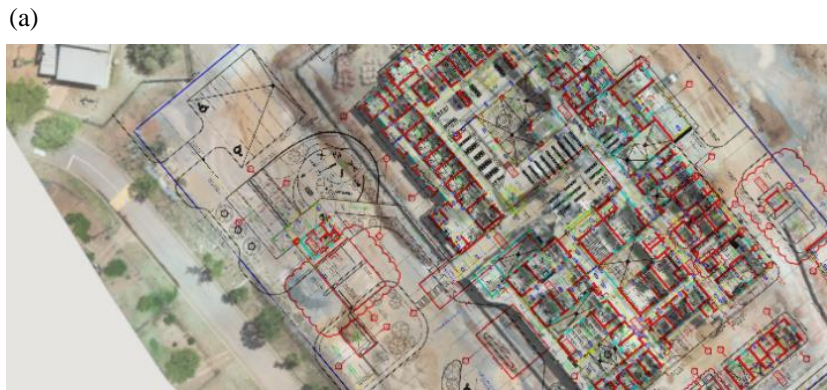
Fig. 2. (a) CAD overlay applied over Orthomosaic map
