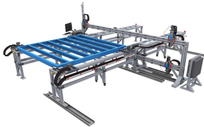
Fig. 5. Automated steel wall framing machine
