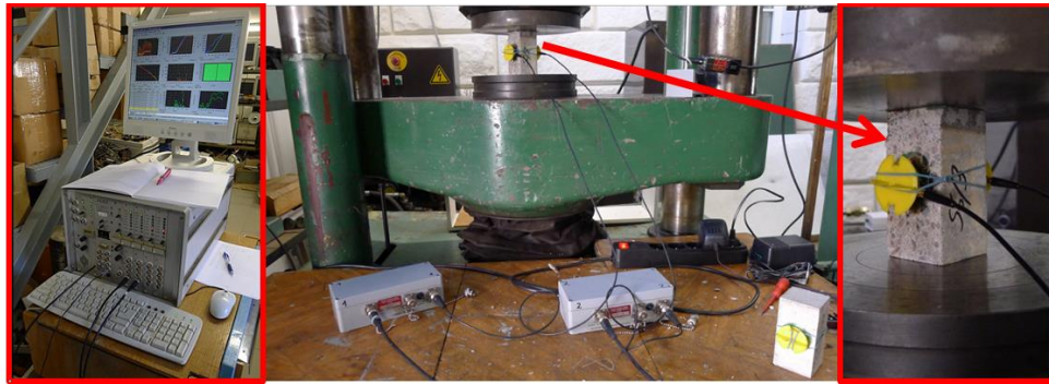
Fig. 3. The stand for testing the failure process using the acoustic emission method.
