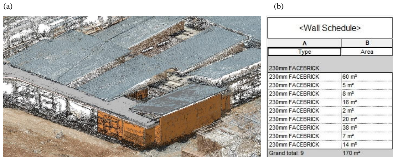
Fig. 5. (a) Walls traced from Point Cloud in Revit 2019 (b) Wall schedule with total area calculated.
