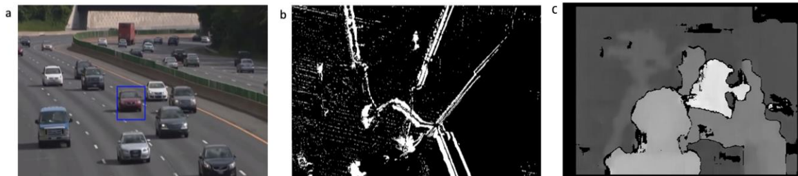
Fig. 3. (a) Meanshift tracker applied to car tracking [30]; (b) background subtraction applied to a video clip [31]; (c) example of stereo vision (depth map) [32].
